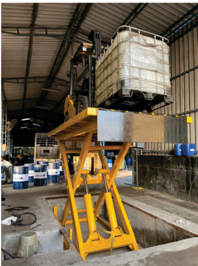
Pit Mounted Scissor Lift Cap : 500 Kg to 20 Ton
