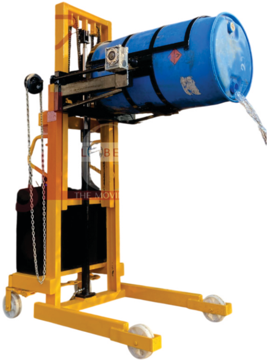
Drum Lifter Tilter (Manual / Semi Automatic / FLP) Lifting Ht - Upto 3500mm
